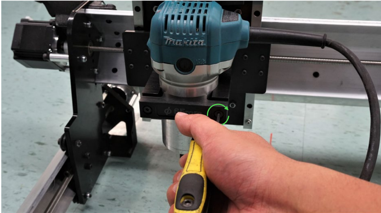
Mount your router with the power cable facing right
