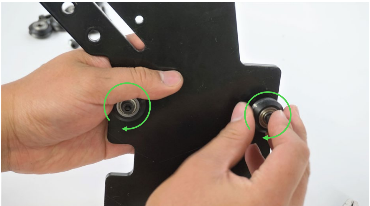
Fasten the wheels to the eccentric nuts, leave these slightly loose for now
