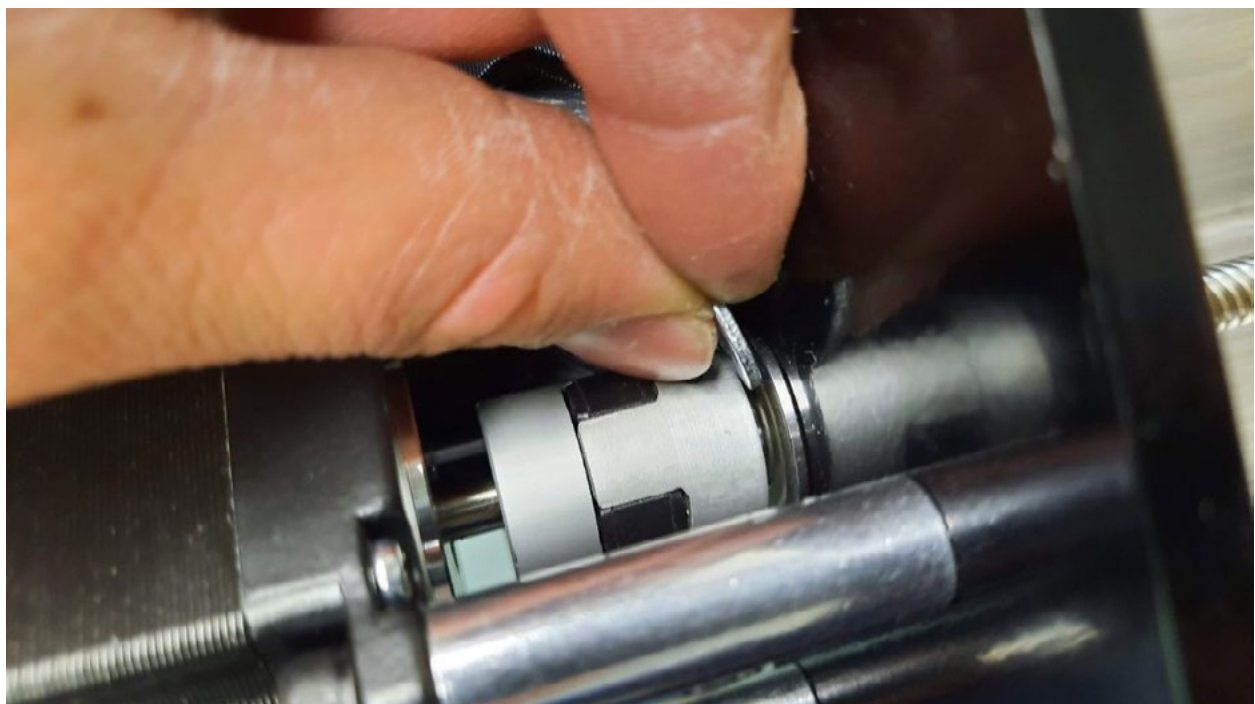
Putting an M8 washer between the coupler and bearing.
