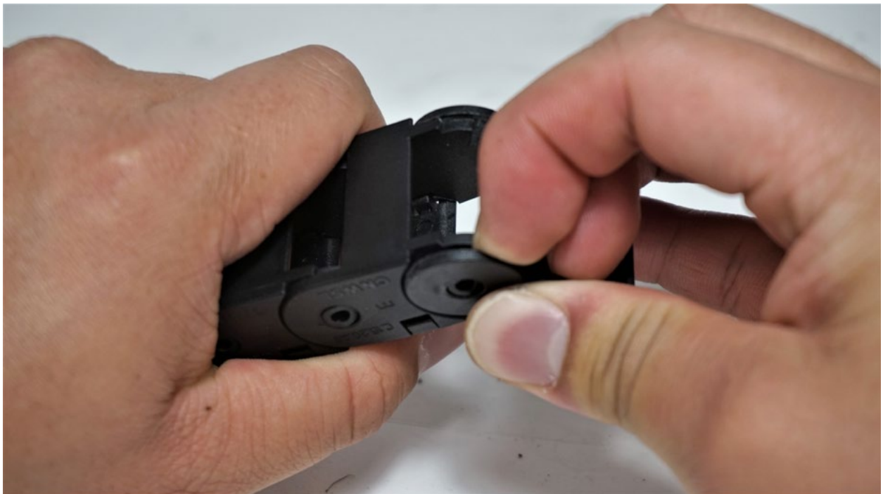
For the hole-type end link, pull on one side of the link then twist it away to separate it
