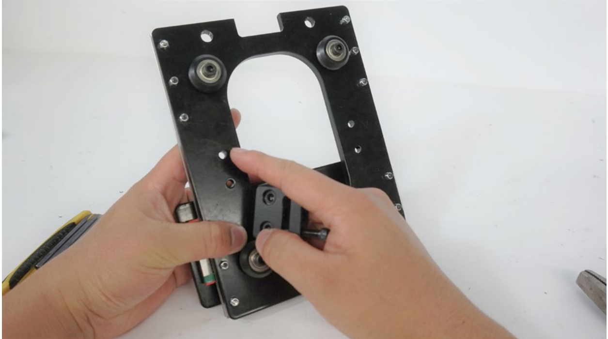
Two holes for mounting the anti-backlash nut block.
