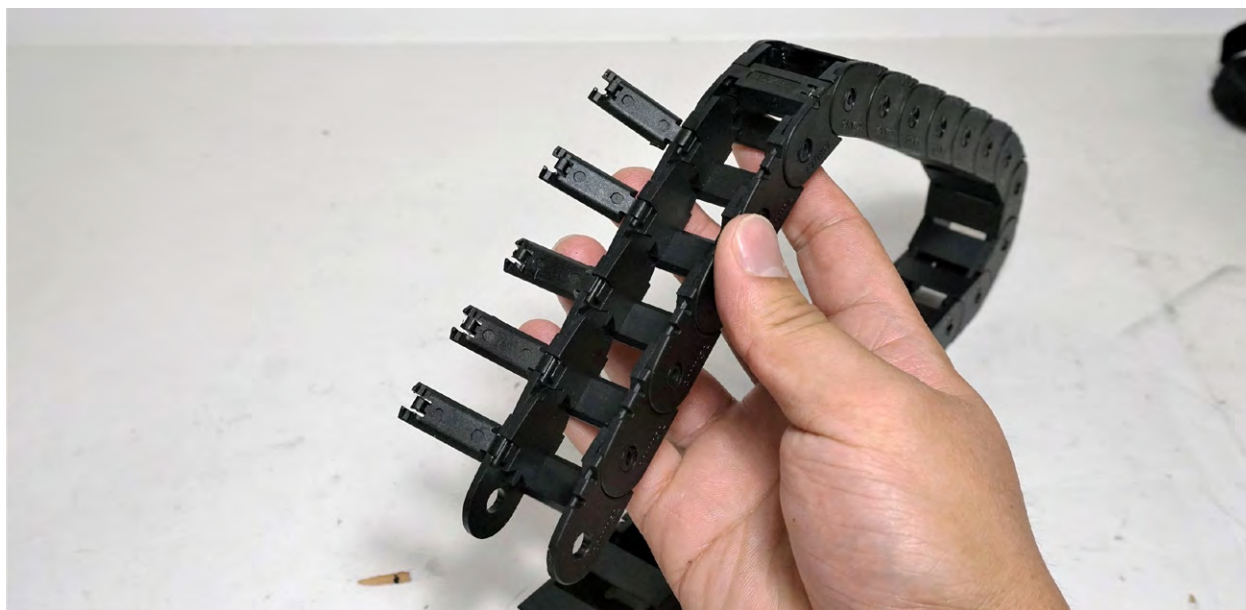
Unclip the tabs on the drag chain
