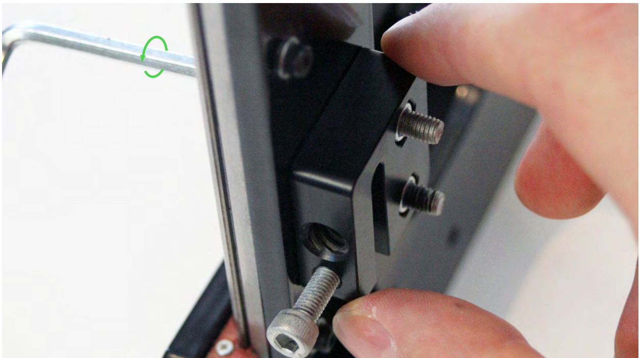
Tighten until snug, but do not overtighten.
