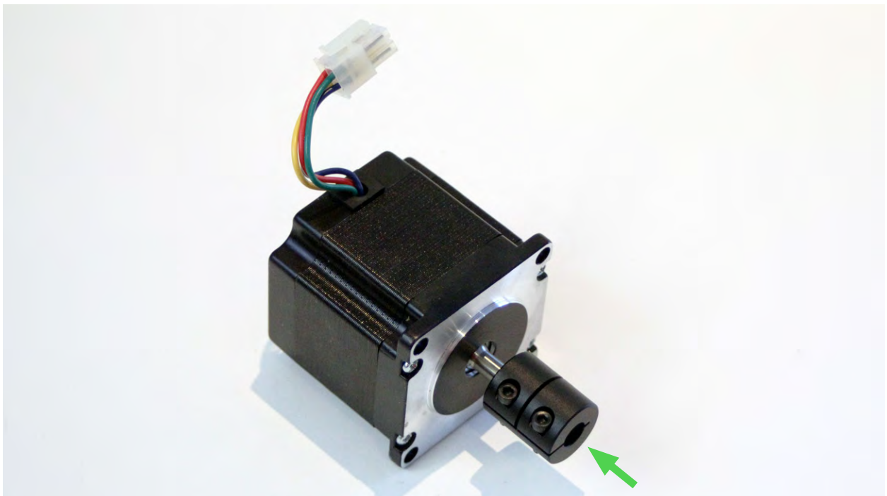
Loosely push the coupler over the motor shaft
