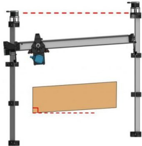
Back feet not aligned (causes skewed cutting)
