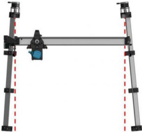
Y-axes aren't parallel to each other (causes machine stress)
