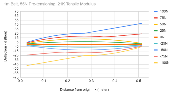
Belt deflection with minimal pre-tensioning (Predicted)
